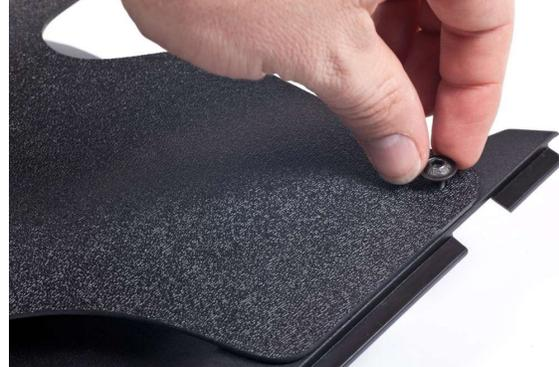
4.) Use the **shorter screws for the rear holes**. Tighten them slightly with your hand first, before you tighten them with a 4mm Metric hex key. All screws do not have to be super tight.
