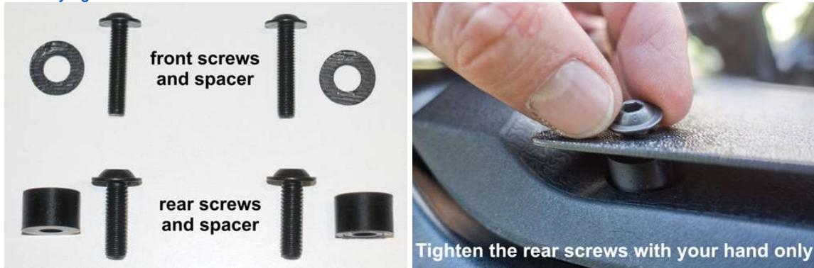
4.) Now use the **longer screws for the front holes**. Tighten them slightly with your hand first. *Note: You need to push down the screw a bit and it also helps when you push down the Forkshield to bring it more into position. The tank cover front nut on the Africa Twin is inside a flexible rubber piece so it might feel a bit strange to get the screw into the nut. This is why you need to push the screw down. You will feel that everything is OK when the screw is inside the nut thread.*
