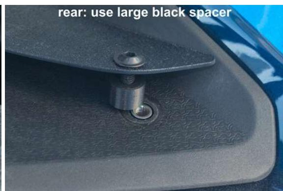
3.) Then attach the SWEGOTECH Forkshield to your bike facing the textured side up by using the **shorter screws for the rear holes FIRST**. (We recommend using Anti-Seize Lubricant on the screw thread to protect the nuts on the gas tank even better). Tighten the screws slightly with your hand only (no tools).
