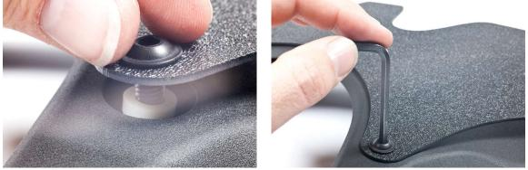
5.) Now also **<u>carefully</u>** tighten the front screws with a 3mm Metric hex key.
