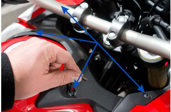
2.) Rear: Place one of the <u>larger</u> spacers <u>above</u> both rear screw holes (left picture) Front: Push one of the <u>smaller</u> spacers completly <u>into</u> both front screw holes and place one black washer on top of it (right picture)
