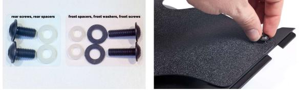
4.) Use the **shorter screws for the rear holes**. Tighten them slightly with your hand first, before you tighten them with a 4mm Metric hex key. All screws do not have to be super tight. **!!! Be careful not overtighten the rear screws to avoid damage on the plastic !!!**
