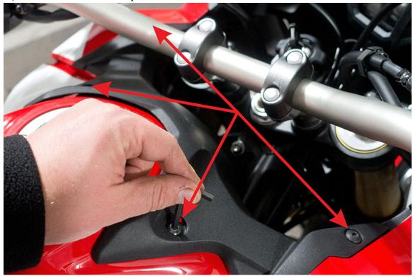
2.) Place the small washers into the front screw holes and the larger Nylon spacers into the rear screw holes on each side
