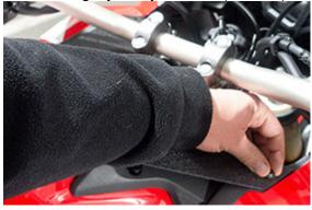
4.) Use the <u>larger screws for the rear holes.</u> Tighten them slightly with your hand first, before you tighten them with a 4mm Metric hex key. <u>Do not overtighten the screws !!!</u>
