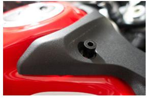
3.) Attach the Forkshield to your bike (textured side to the top) by using the **smaller screws for the front holes**. Tighten the screws slightly with your hand (no tools)
