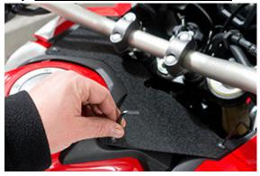
5.) Tighten the front screws with a 3mm Metric hex key now **Note:** The front screws should **not** be super tight
