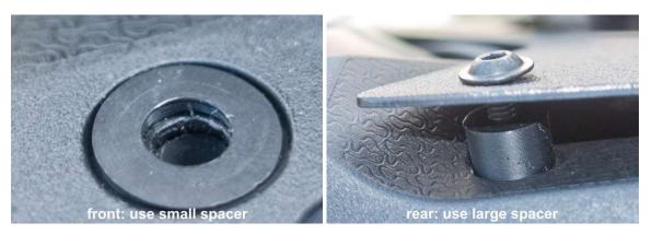
3.) Then attach the SWEGOTECH Forkshield to your bike facing the textured side up by using the **shorter screws for the rear holes FIRST**. (We recommend using Anti-Seize Lubricant on the screw thread to protect the nuts on the gas tank even better). Tighten the screws slightly with your hand only (no tools).
