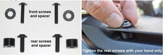
4.) Now use the <u>longer screws for the front holes.</u> Tighten them slightly with your hand first. Note: You need to push down the screw a bit and it also helps when you push down the Forkshield to bring it more into position. The tank cover front nut on the Africa Twin is inside a flexible rubber piece so it might feel a bit strange to get the screw into the nut. This is why you need to push the screw down. You will feel that everything is OK when the screw is inside the nut thread.
