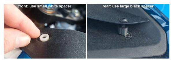
3.) Then attach the SWEGOTECH Forkshield to your bike facing the textured side up by using the **shorter screws for the rear holes FIRST**. (We recommend using Anti-Seize Lubricant on the screw thread to protect the nuts on the gas tank even better). Tighten the screws slightly with your hand only (no tools).
